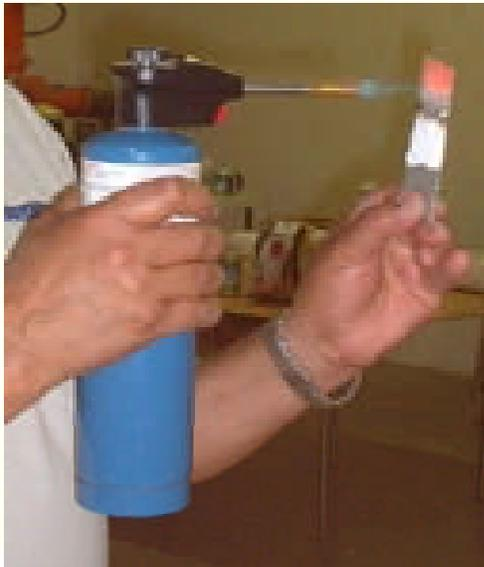
The metal is coated with MULTICERAMICS in a one inch strip in the middle of one side only, one extreme of the metal strip is heated with this butane torch to 1500F. This would be impossible to be held if the coating did not stop the conduction through the surface of the metal. MULTICERAMICS really works! This test could not be performed with regular paint, nor with fiberglass, foam, or other insulators.
