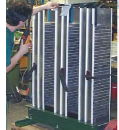
Partially assembled reactor with PolyGap™ core
